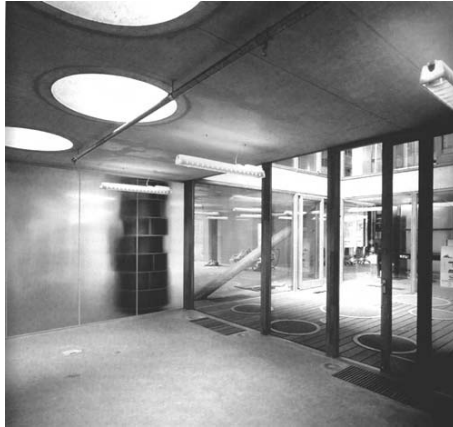
Figure 8.6 Floor height domes to provide sufficient daylight
